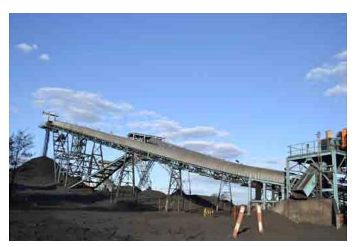
The conveyor belt that moves coal from MCM to the adjacent Morupule B Power Station
