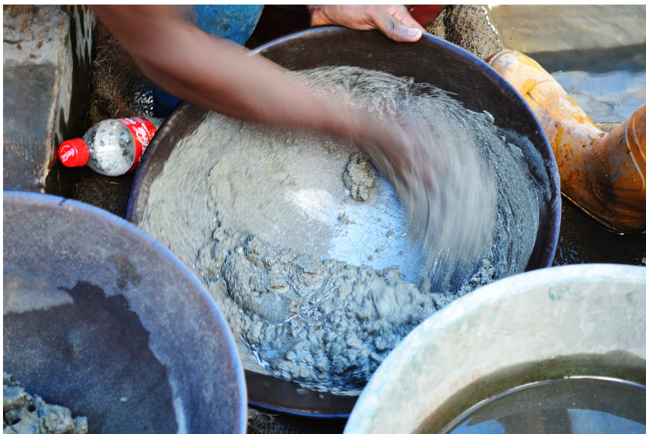
A miner at the Nsangano operation uses mercury (in the Coca-Cola bottle) to extract gold from the crushed ore
