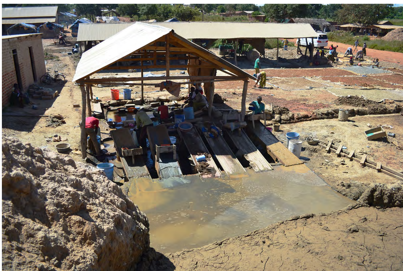
The waste from the Swiss boxes that is not processed using mercury is piled up in walls of sludge. Workers shovel this waste to other processors, some of whom use cyanide to extract gold
